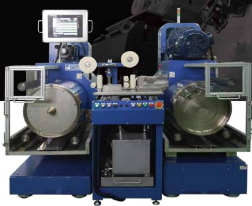
Drawing element wires of various materials produced in welding processes with stable lower tension. Supporting a wide range of element wire diameters (fine or thick) and types (soft or hard). Fluctuation in tension during acceleration and deceleration has been extremely reduced with precise inertia compensation using our high-precision control technology.
